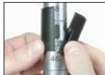
Snap sleeve around numbered post.
